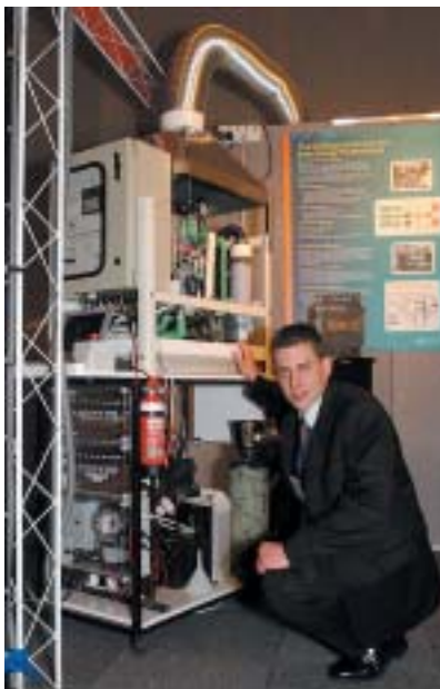
Engineer, Ben McQueen, with IRL's demonstration fuel cell system; this alkaline fuel cell system supplied 400 W of energy to 12 spotlights.
