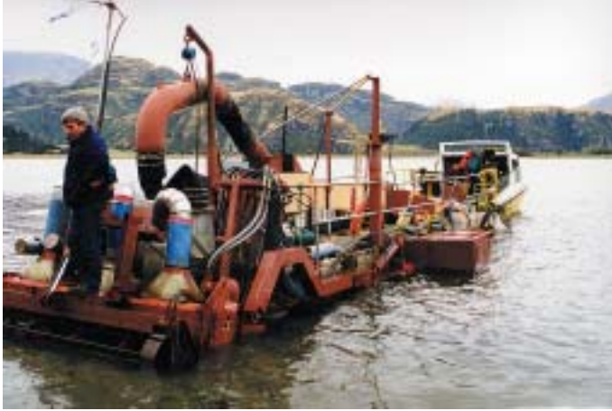
A weed harvester mechanically removes weeds from the edges of Lake Wanaka. Photo: John Clayton, NIWA
