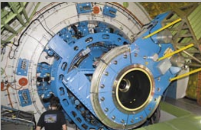
↑ A technician examines the instrument mounting structure and bulkhead of the German-built infrared telescope installed in NASA's SOFIA airborne observatory.
