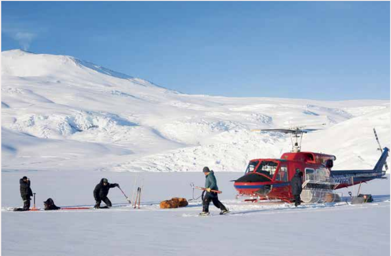
Above: With Mount Erebus in the background, Dr John Stodt, Phil Wannamaker, and Graham Hill set up a magnetotelluric sounding site in the Windless Bight area of Ross Island. Image: Danny Uhlmann
