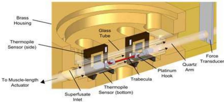
Cut-away diagram of the microcalorimeter.
