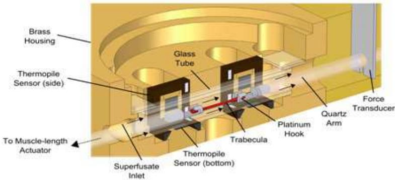
Cut-away diagram of the microcalorimeter.
