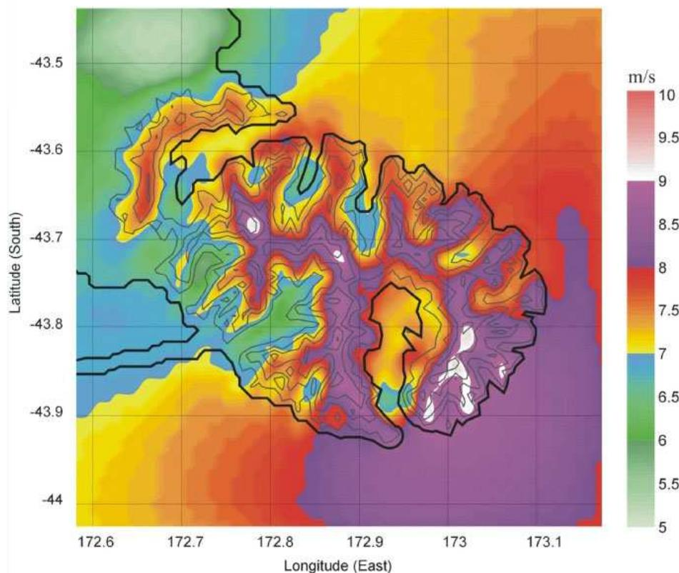
Figure 1. Map of the mean wind speed over Banks Peninsula in 2002 (50 m above ground at a resolution of 800 m), from the collaboration between Canterbury University and Connell Wagner.
